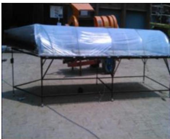
**Fig. 1: Solar tunnel dryer**
