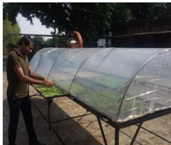
**Fig. 2: Drying of mint leaves in solar tunnel dryer**
