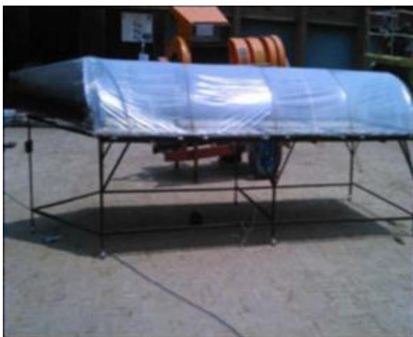
**Fig. 1: Solar tunnel dryer**
